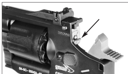
A valve releases CO 2 when the hammer strikes the transfer bar between the valve's release pin and the hammer's front face.
